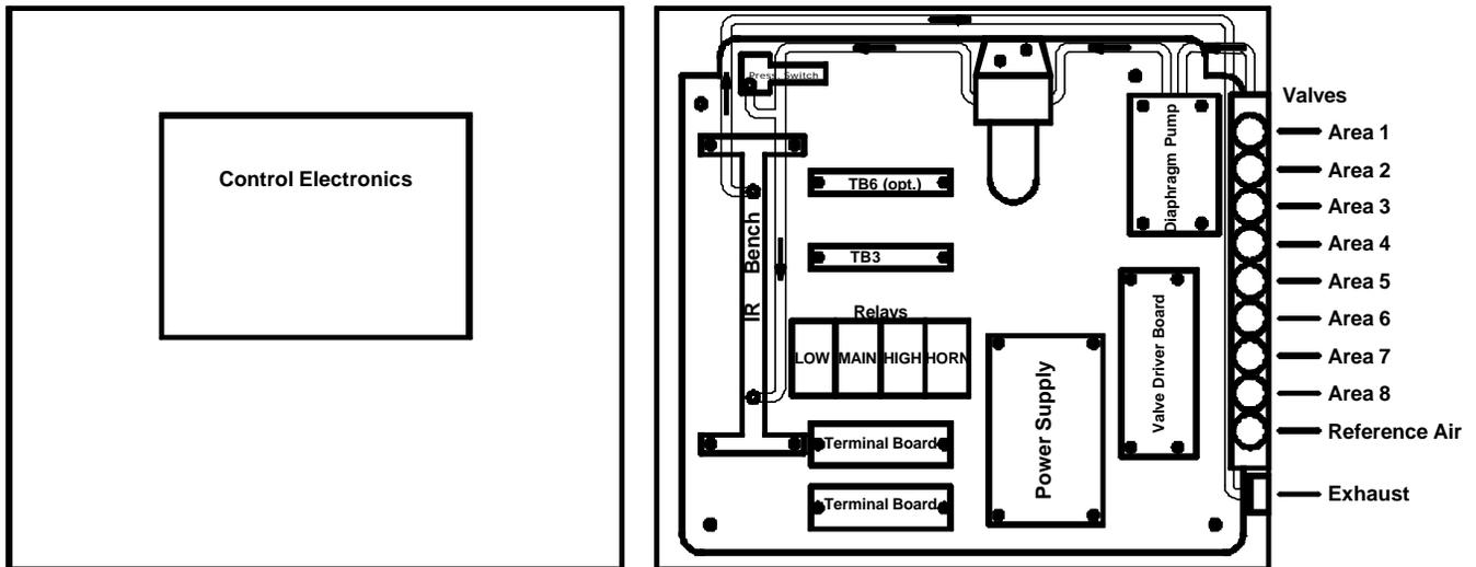
Figure 6. Parts Diagram
