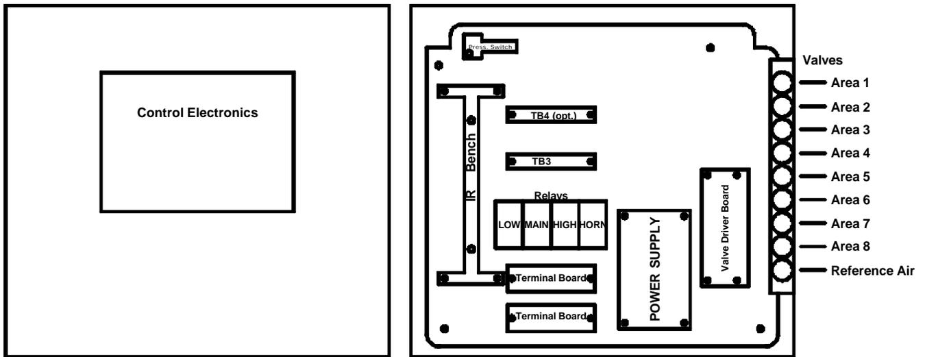
Figure 4 Control Electronics Diagram
